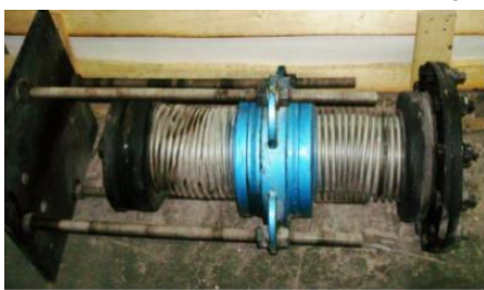
Fig. 7. Primary sample of contractable viscous dashpot
