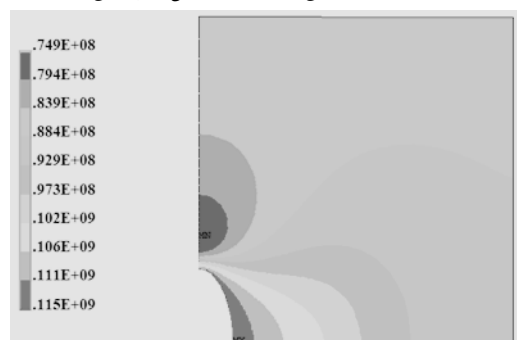
Fig. 13. von Mises stress distribution over the optimized hole using evolutionary structural optimization and nonlinear analysis
