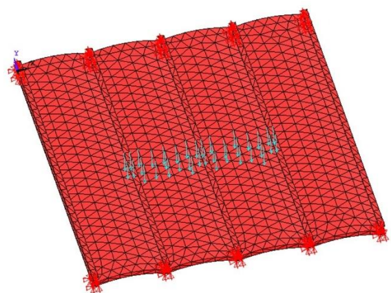
Fig. 11. The modelled jack arch roof for calibration
