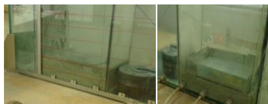
Fig. 5. Placement of a can and compaction of sand in it
