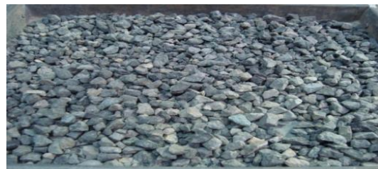
Fig. 4. Gravel used in stone column
