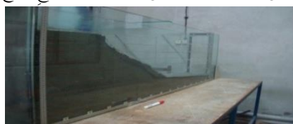
Fig. 9. Completed rupture of saturated unreinforced slope
