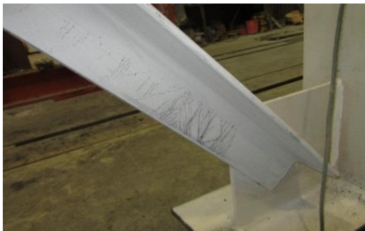
Figure 16: The brace buckling in the laboratory
