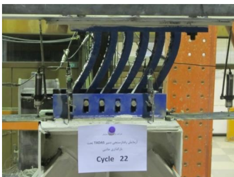
Figure 12: Damper deformation in the laboratory
