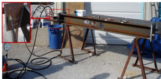
Fig. 2. Prestressing system used to simulate axial load [6]
