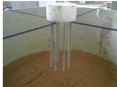
Figure (6): Solidification of cap and micro piles in the third group
