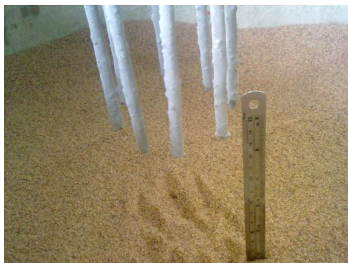
Figure (4-b): A view of micro piles coated with glue
