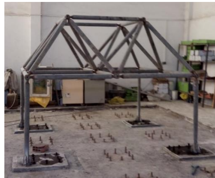
Fig. 2. The double layer Grid made in a Laboratory
