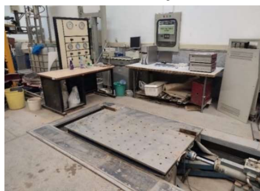
Fig. 2. Shaking table of Tehran university
