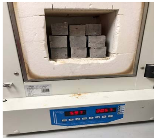
Fig. 2. The arrangement of the samples in the furnace under the heat of 600 degrees
