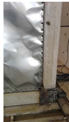
Fig. 12. No rupture of the web plate and no separation from the connecting plate
