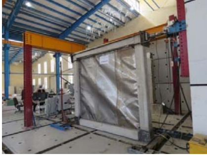
Fig. 10. Sample after loading up to 2.02% displacement
