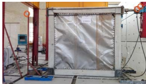
Fig. 6. The displacement position of the gauges
