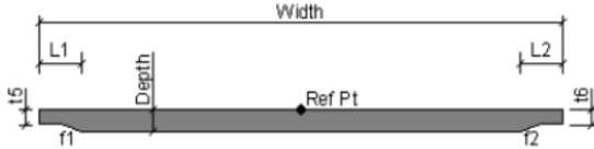
Fig. 4. Bridge deck detail
