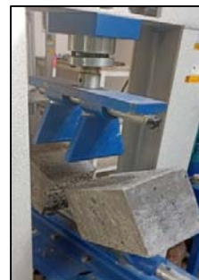
Fig. 2. Concrete sample after failure in flexural strength test.
