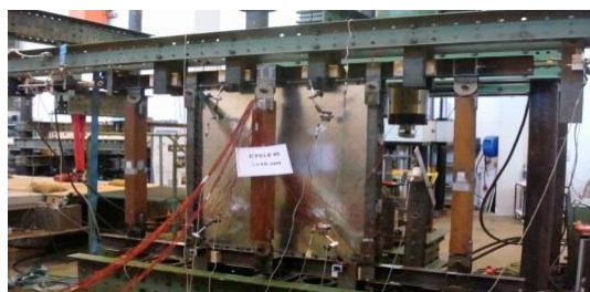
Fig. 8. Laboratory model of semi-supported steel shear wall [14]
