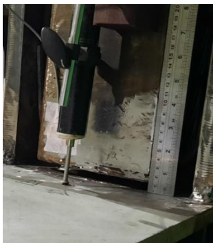
Fig. 12. Measuring the opening of the connection in the drift 3%
