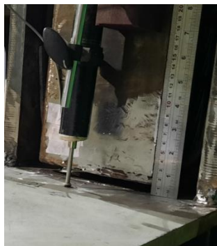
Fig. 12. Measuring the opening of the connection in the drift 3%
