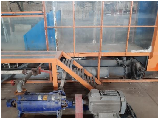
Fig. 2. A view of the flume and jet system
