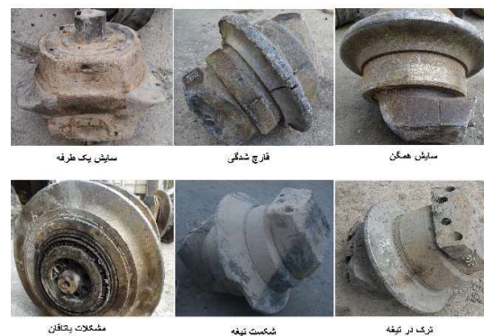
Fig. 15. Examples of disc cutter failures pattern in Lot 2 of the Kani Sib tunnel
