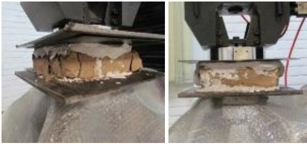
Fig. 5. Compressive strength test on adobe sample
