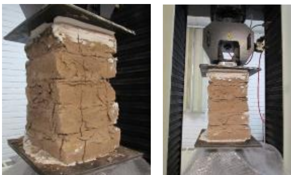
Fig. 6. Compressive strength test on adobe prism
