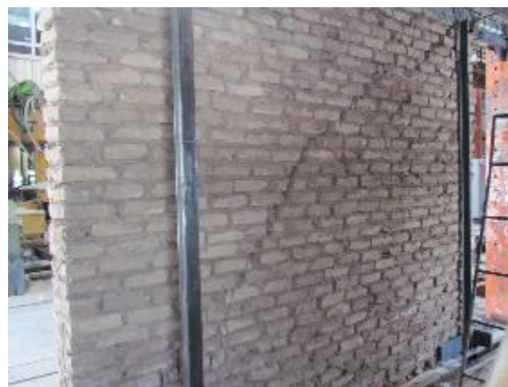
b) Back view of the cracking in the wall Fig. 12. Overall view of the wall at the end of the test
