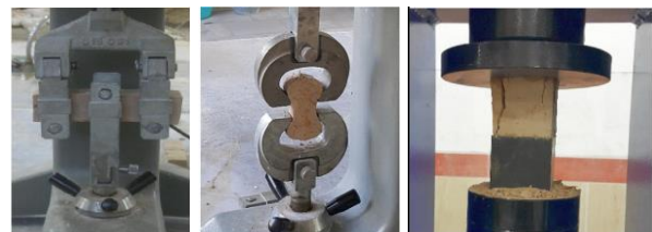
Fig. 4. Set-up for compressive, tensile and flexural strength tests of clay mortar
