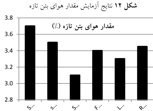
Figure 12. The results of testing the air content of fresh concrete
