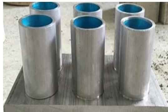
Fig. 6. Concrete cylindrical molds
