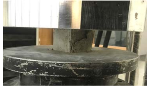
Fig. 4. Cubic sample in uniaxial compressive test to determine concrete mix design
