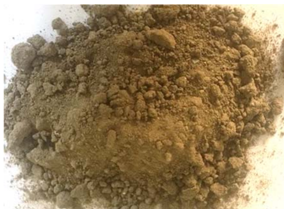
Fig. 1. Fine sand used in concrete mix
