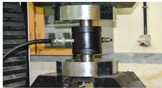
Fig. 10. Triaxial compression test using a Hook cell
