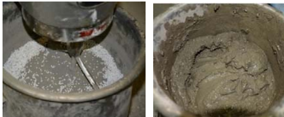
Fig. 7. EPS concrete mixing design process
