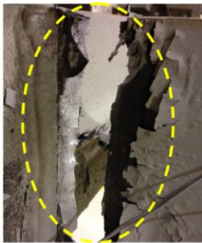
Fig. 6. Cyclic diagram of force-displacement and failure mode of direct welded connection sample [1]
