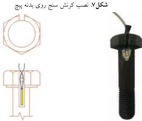
Fig. 7. Installation of strain gauges on bolt shanks
