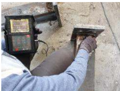
Fig. 2. CJP Ultrasonic Weld Test
