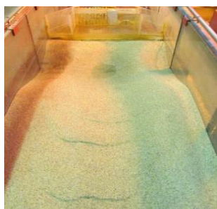
Fig. 3 Downstream view of scouring
