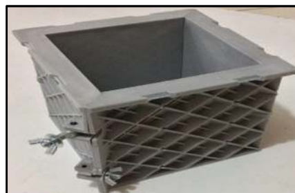
Fig. 3. The used template in making the product to check the sealing rate
