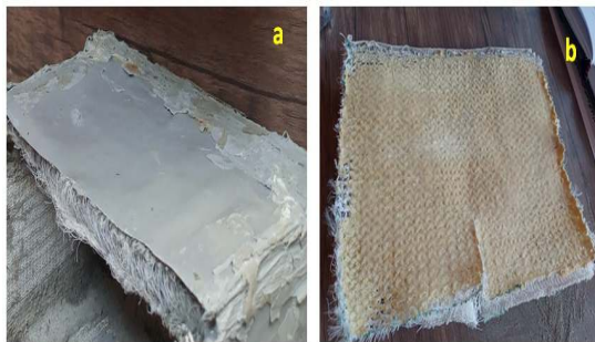
Fig. 4. The produced Concrete canvas both casting method and with geo-membrane.
