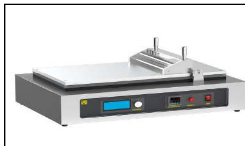
Fig. 2. Dr.Blade device for concrete canvas covering
