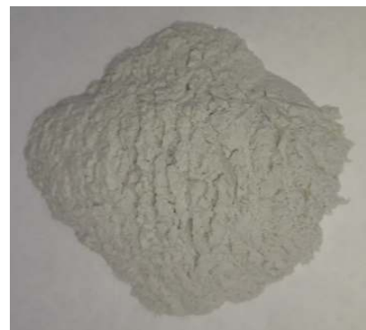
Fig. 3. Glass powder used to replace cement
