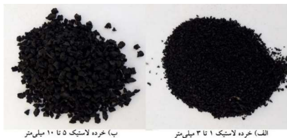
Fig. 1. Rubber crumbs used in concrete
