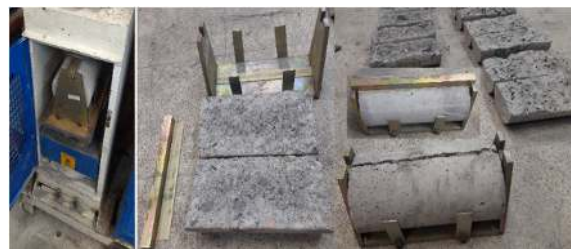
Fig. 7. Process and tools for tensile testing
