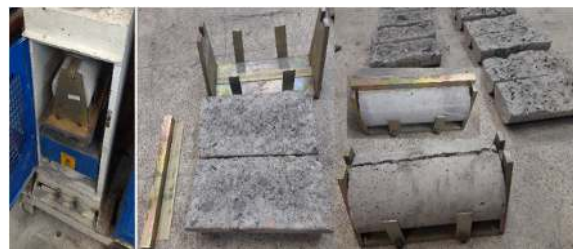
Fig. 7. Process and tools for tensile testing
