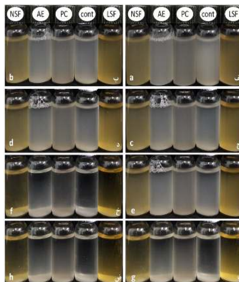
Fig. 8. The effect of surfactant on the HNT dispersion; a) initial state, after b) 15 min c) 50 min d) 2 hours e) 2 hours and 45 min f) 20 h and 30 min g) 25 h h) 31 h and 40 min
