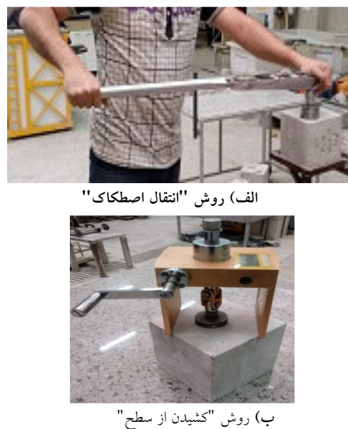
Fig. 3. Evaluation of the compressive strength of mortars
