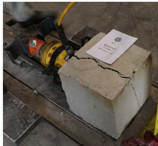
Fig. 9. Picture of split concrete (P25S-2) after test
