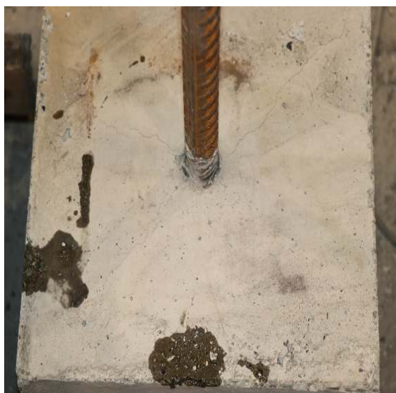
Fig. 7. Picture of pulled out rebar (P25S1)
