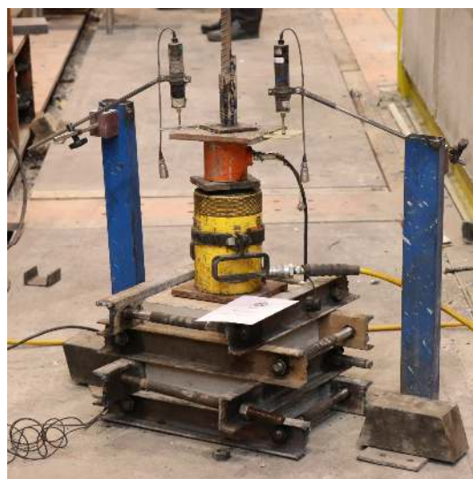
Fig. 5. Test setup for pullout test of confined concrete
