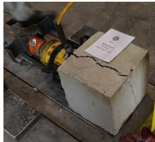
Fig. 9. Picture of split concrete (P25S-2) after test
