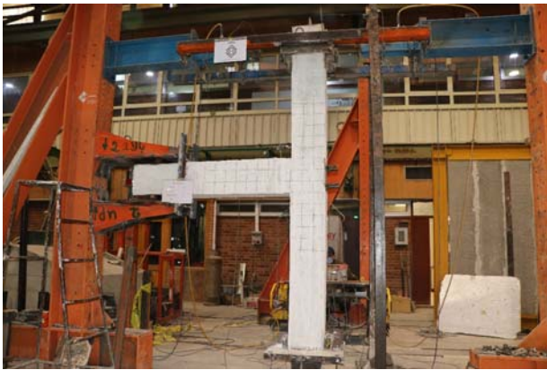
Fig. 8. Test setup of specimens and out of plane lateral support
