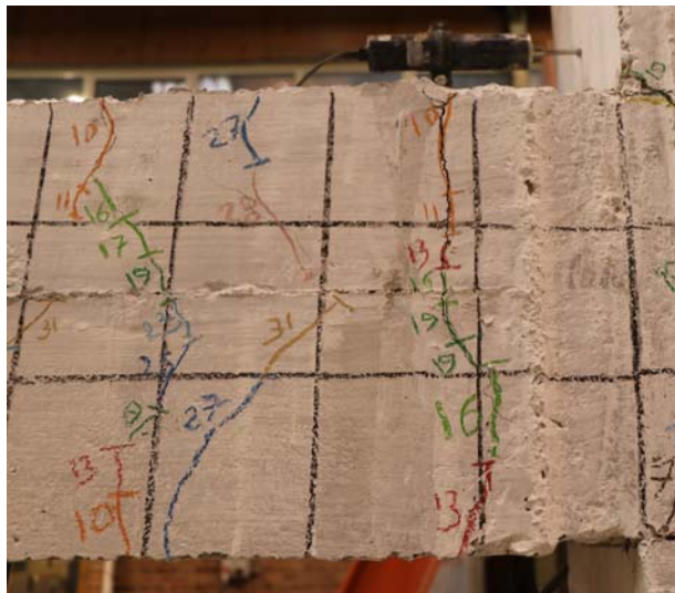
Fig. 12. Plastic hinge of TNN sample at 3.5% drift
