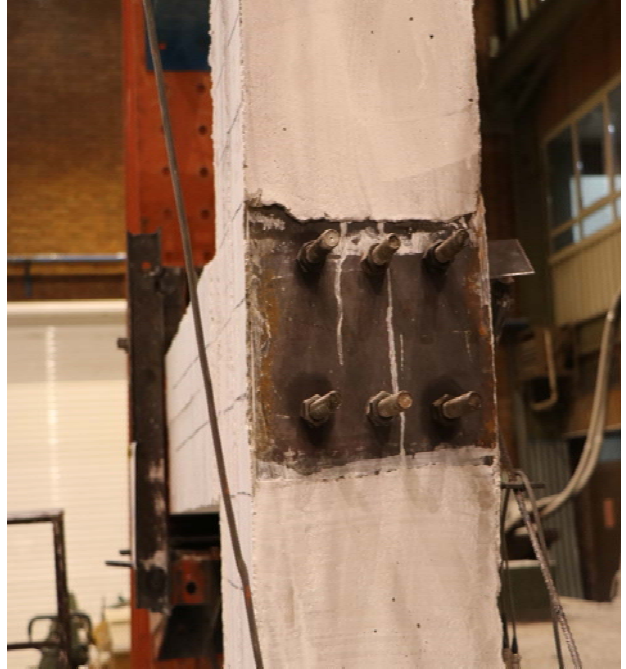
Fig. 2. Anchorage of rebars on rear side of column of TNN sample
