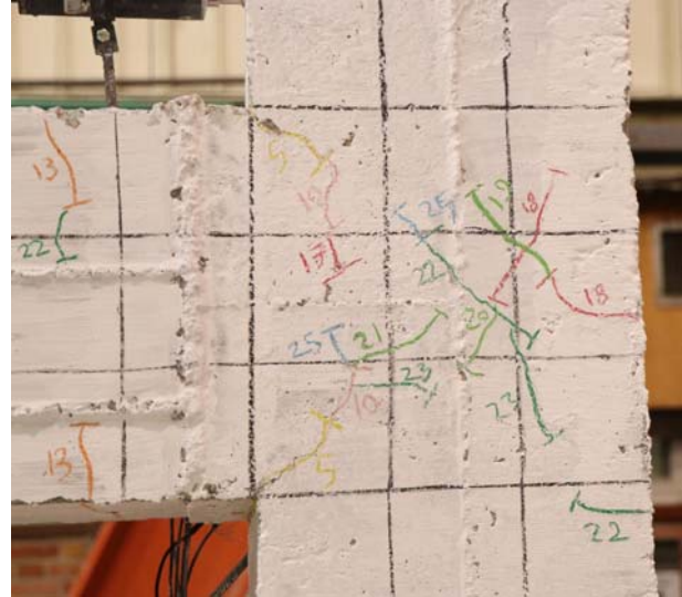
Fig. 9. TDN sample at 2.2% drift
