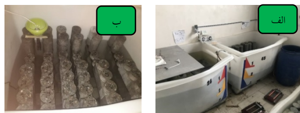
Fig. 3. a) Simulators immersion environment and tides, b) placement of the samples in terms of immersion and tide.
