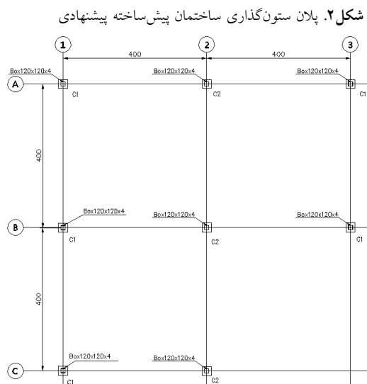
Fig. 2. Column plan of the proposed prefabricated building
