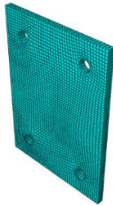
Fig. 18. Mesh pattern of the perforated plates with an element size of 4 mm
