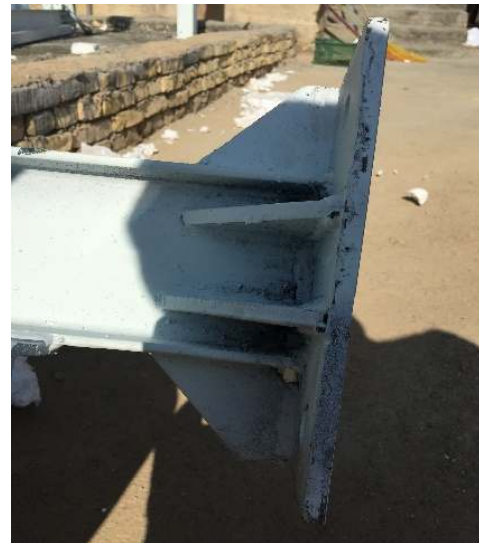
Fig 8. A close-up view of the fabricated beam-to-end plate connection
