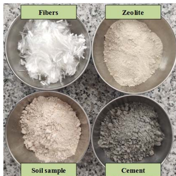
Fig. 2. A view of soil, cement, zeolite and fibers used in this study
