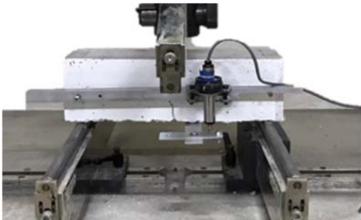
Fig. 13. Detail of Flexural specimens and LVDTs
