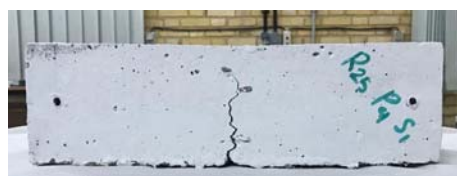
Fig. 15. Schematic of cracking of flexural specimens
