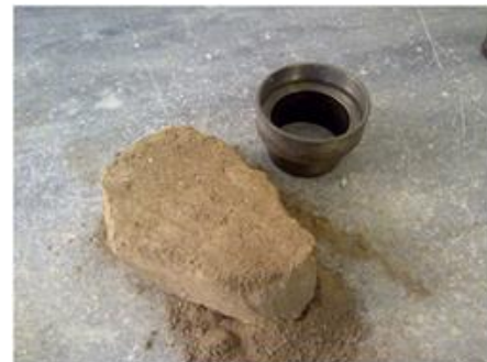
Fig. 5. Cut piece from obtained in-situ intact sample
