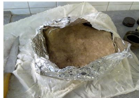
Fig. 4. In-site intact block sample
