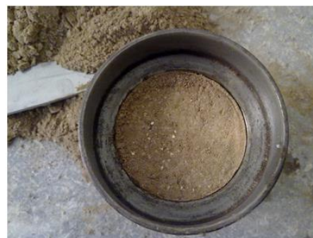
Fig. 6. Taking an intact sample with a sampler
