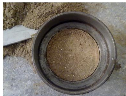
Fig. 6. Taking an intact sample with a sampler
