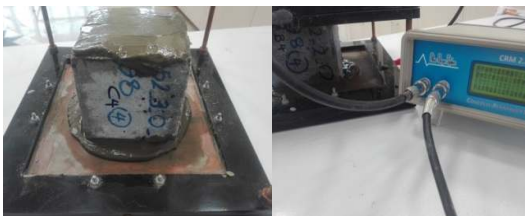
Fig. 4. Electrical resistance test
