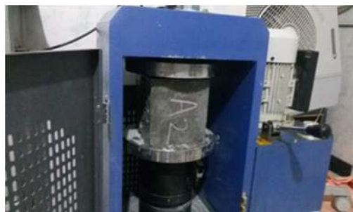
Fig. 5. Compressive strength test according to ASTM C 109 standard
