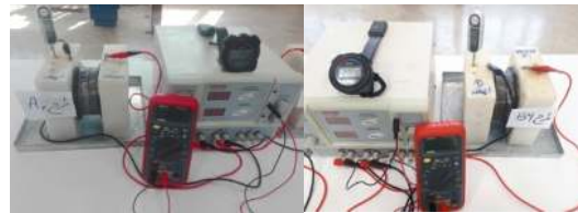
Fig 3. RCPT test according to ASTM C1202 standard
