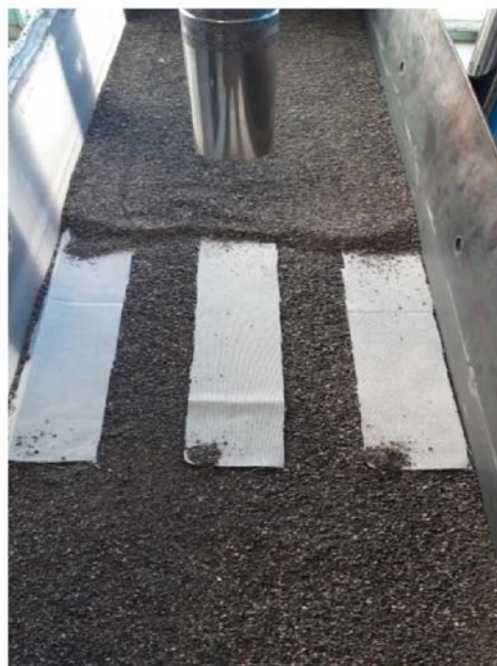
Fig. 4. Placement of the geotextile strips in the model
