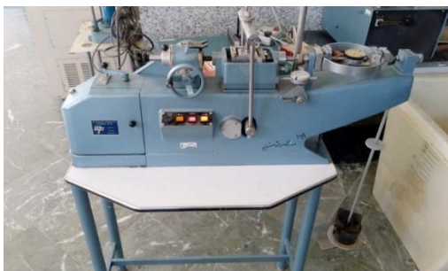
Fig. 5. Direct shear machine used in this project
