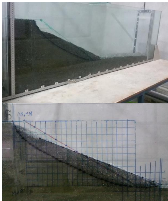
Fig. 6. First model failure after 380 minutes
