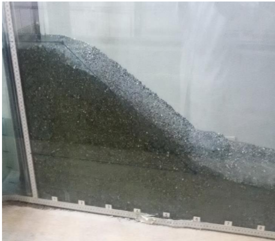
Fig. 10. Second model failure after 240 minutes
