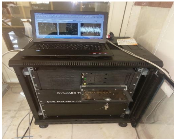
Fig. 3. System for receiving, analyzing and sending data with software
