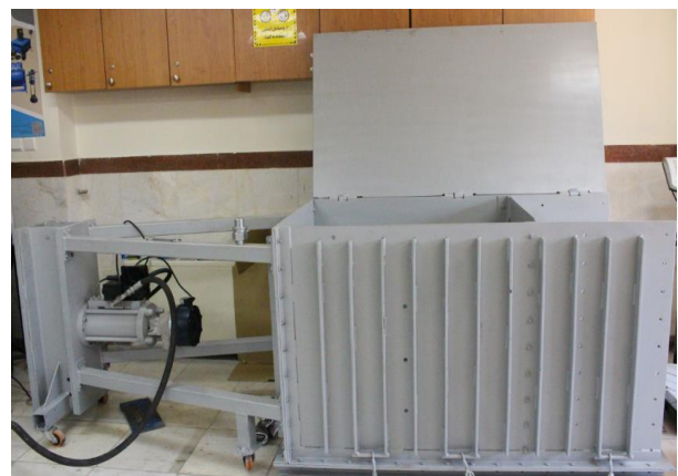
Fig. 2. General shape of the nail pullout set
