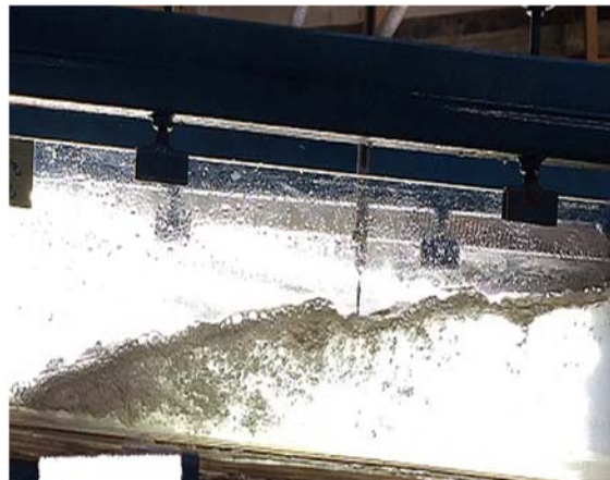
Fig. 5. Side-view of a hydraulic jump
