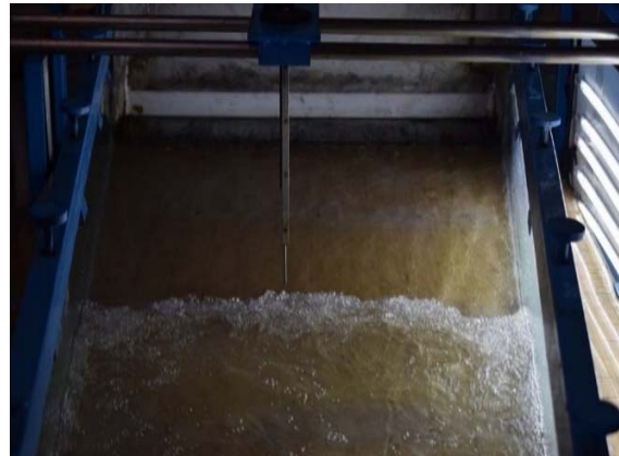
Fig. 4. Uniformity of hydraulic jump front by regulating inflow gate
