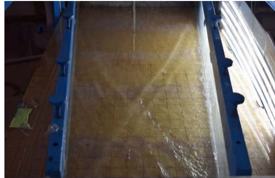
Fig. 3. Collision of oblique waves at the centerline of the inclined convergent channel
