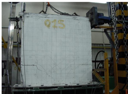
Fig. 7. Cyclic loading on specimen with dimensions 120x120 cm
