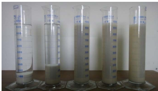
Fig. 4. Sedimentation of mixtures of bentonite-TSP, (from right to left: 0, 1, 2, 5, 10% TSP).
