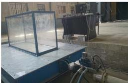
Fig. 1. Model container on the shaking table
