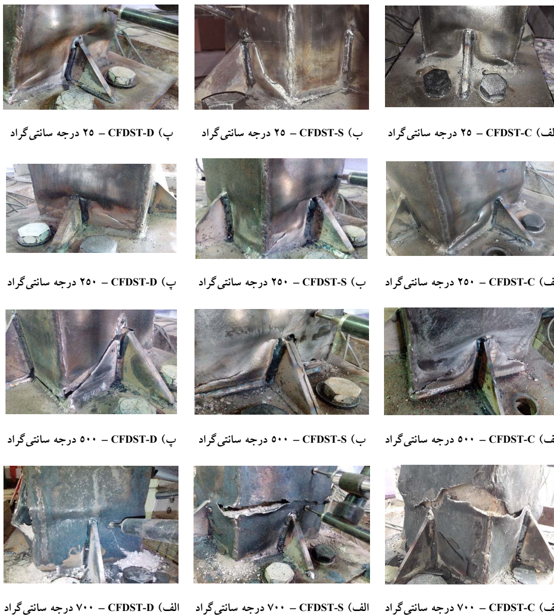
Fig. 10. Modes of rupture of columns at different temperatures
