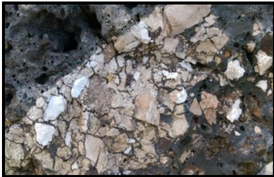
Fig. 6. The microscopic image showing cement paste, anhydride and calcite from a mixed sample with various materials
