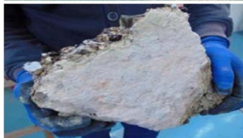
Fig. 5. Sample F3 after fire resistance test in the furnace
