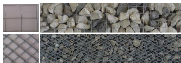
Fig.2. Grids used to make gabion spur dike
