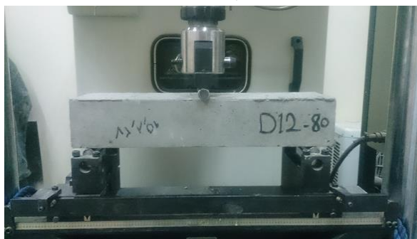
Fig. 4. Test of fatigue life of concrete samples
