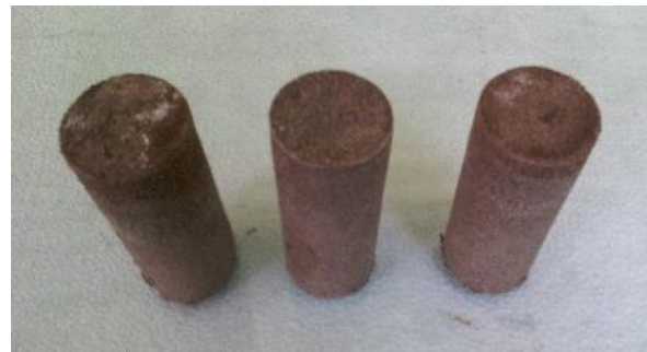
Fig. 5. Prepared samples for unconfined pressure test
