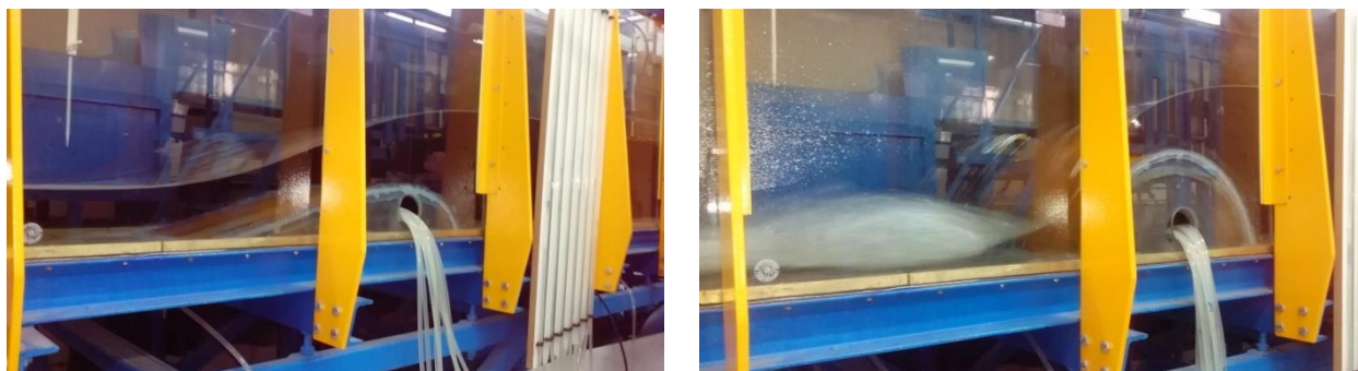
Fig. 15. Flow behavior over a circular-crested weir compared to that over a streamlined weir, with \lambda = 0.25
