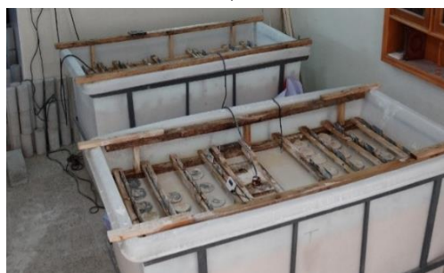
Fig. 2. a) Specimens in the container; b) Preparing an alkaline environment (container 1 & 2)
