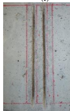
Fig. 1. a) Specifications of the specimens used; b) EBR method; c) EBROG method
